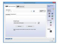
(Note) Enter the Digital Output(Optical) screen to configure further settings if you use the S/PDIF Out connector(s) on the back panel for digital audio output or enter the Digital Output screen if you use the internal S/PDIF Out connector (SPDIF\_O) for digital audio output.
