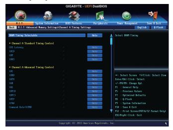
This sub-menu provides memory timing settings for each channel of memory. The respective timing setting screens are configurable only when **DRAM Timing Selectable** is set to **Quick** or **Expert**. Note: Your system may become unstable or fail to boot after you make changes on the memory timings. If this occurs, please reset the board to default values by loading optimized defaults or clearing the CMOS values.
