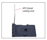
Step 1: Completely lift up the APU socket locking lever.
