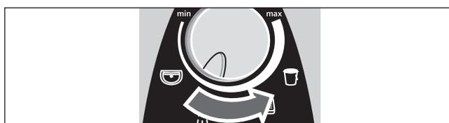
If a higher temperature for a completely opened warm water tap is not achieved, more water flows than the flow-through heater can warm as a result its performance capabilities. In this case, the warm water tap must be closed somewhat.
